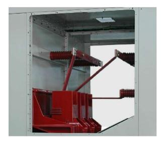
Bus bar compartment contains high conductivity tin Plated or insulated flat rectangular copper bars of proper current carrying cross section supported by epoxy resin cast insulators which are rigid enough to with stand all thermal and electrodynamics thermal stress. Flat tee off connections join the Bus bar directly to the contact spouts of individual feeder
